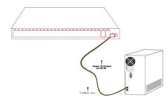
This cable is used to connect the CLI port of switch to the external monitoring end device. It has an RJ45 plug and a 9-pin plug (DB9). The RJ45 plugs into the CLI port socket of the 5236TG28 switch.
