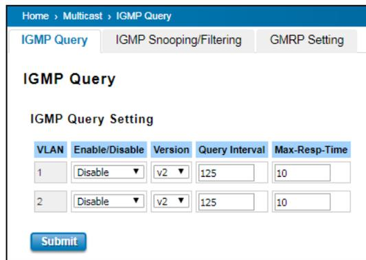
The screenshot shows the 'IGMP Query' configuration page. It has tabs for 'IGMP Query', 'IGMP Snooping/Filtering', and 'GMRP Setting'. Under 'IGMP Query Setting', there is a table with columns: VLAN, Enable/Disable, Version, Query Interval, and Max-Resp-Time. Two rows are visible for VLANs 1 and 2, both with 'Disable' selected, 'v2' version, '125' interval, and '10' max response time. A 'Submit' button is at the bottom.
