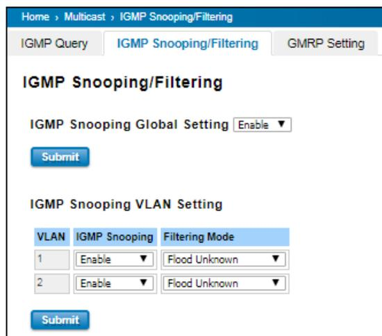
The screenshot shows the 'IGMP Snooping/Filtering' configuration page. It has tabs for 'IGMP Query', 'IGMP Snooping/Filtering', and 'GMRP Setting'. Under 'IGMP Snooping Global Setting', there is a dropdown menu set to 'Enable' and a 'Submit' button. Under 'IGMP Snooping VLAN Setting', there is a table with columns: VLAN, IGMP Snooping, and Filtering Mode. Two rows are visible for VLANs 1 and 2, both with 'Enable' selected and 'Flood Unknown' filtering mode. A 'Submit' button is at the bottom.
