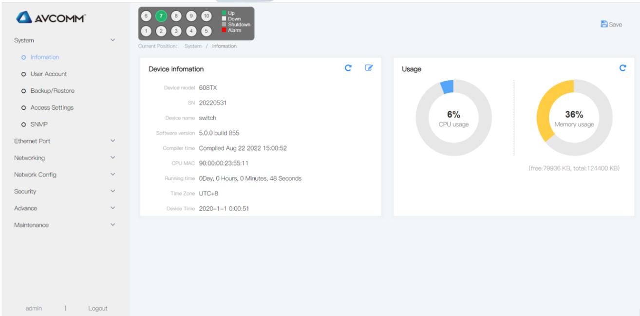
The screenshot shows the AVCOMM web interface. At the top, there is a navigation bar with the AVCOMM logo and a status bar with buttons for Up, Down, Shutdown, and Alarm. Below the navigation bar, there is a sidebar menu with categories like System, Ethernet Port, Networking, Security, Advance, and Maintenance. The main content area is divided into two sections: "Device information" and "Usage".
