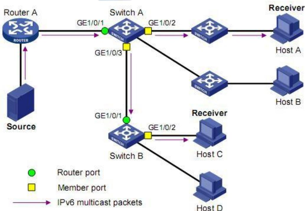
In conjunction with the above diagram, introduce the port concepts associated with MLD Snooping.
